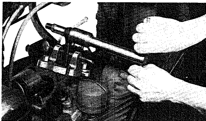
ILLUS. 33 INSTALLING NEW ROD BUSHING
