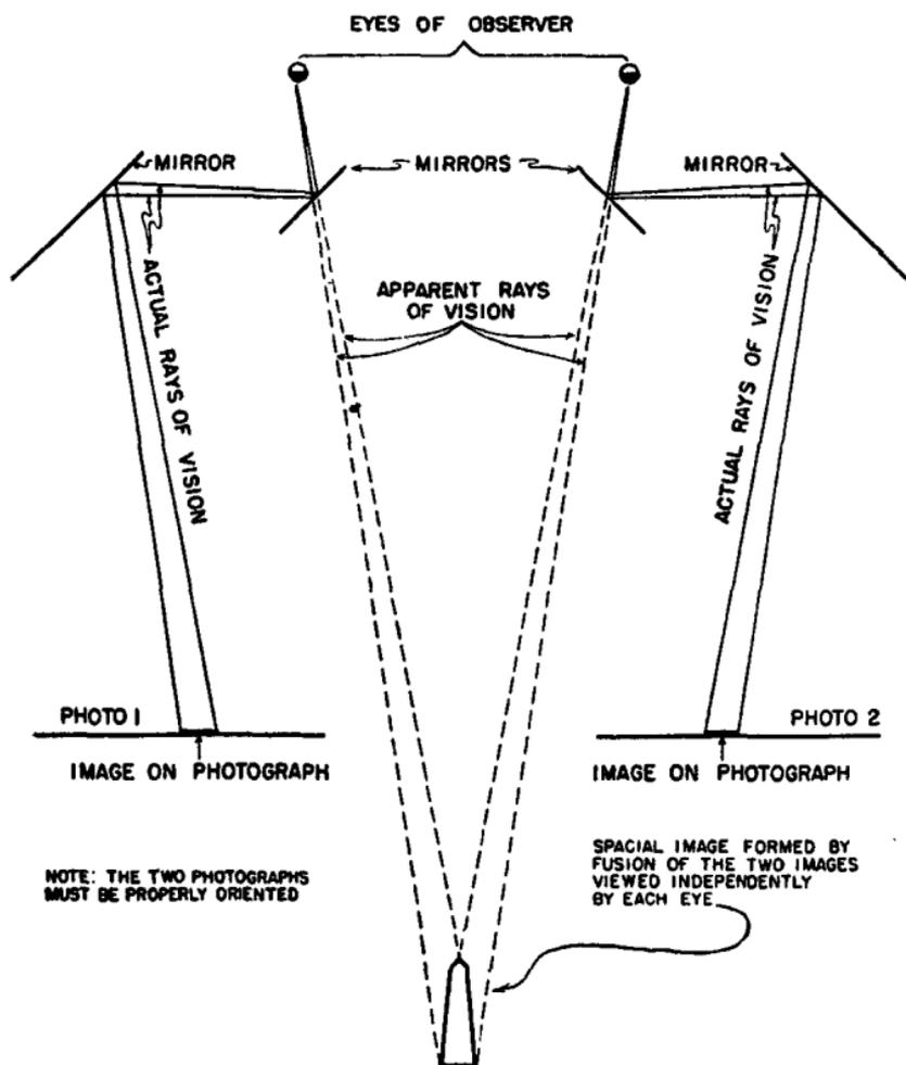
FIGURE 8.—Diagram showing stereoscopic perception.
