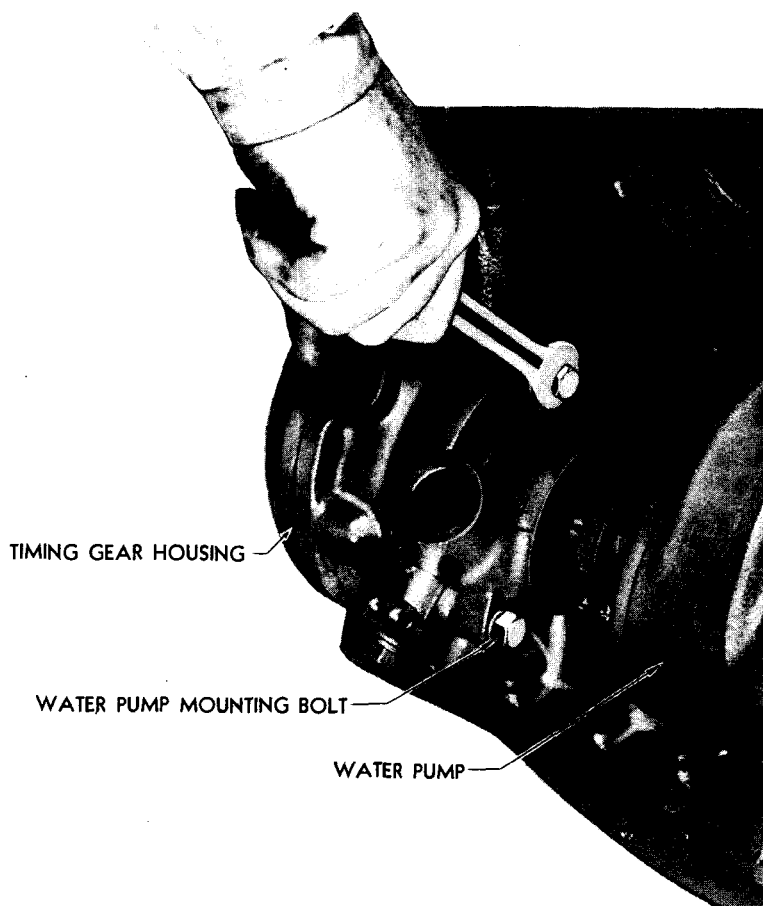
Figure 47—Removing Water Pump Assembly
