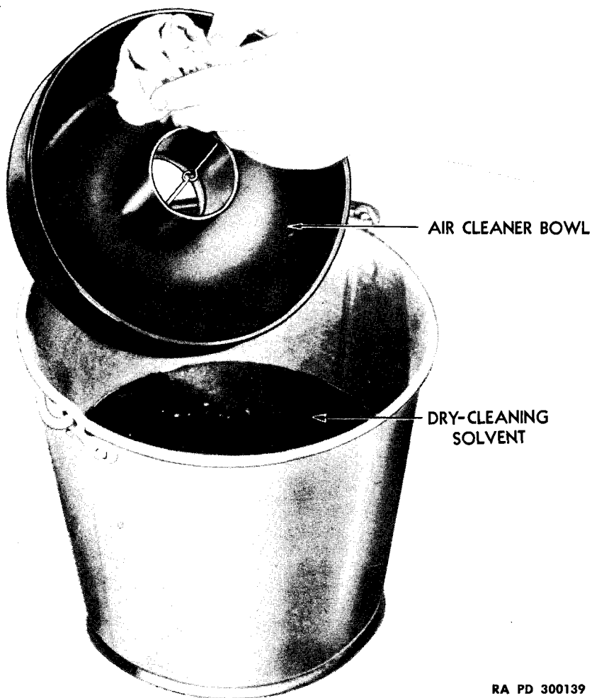
Figure 45—Cleaning Air Cleaner Bowl
