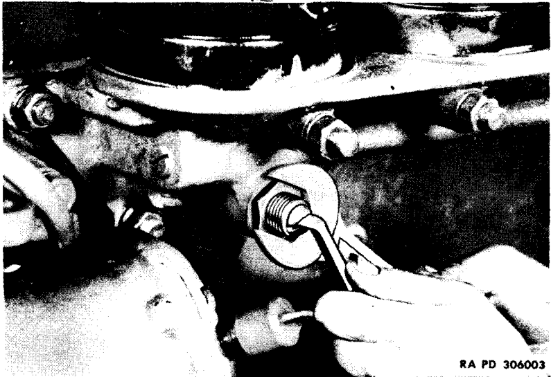
Figure 39—Adjusting Oil Pressure, Using Screwdriver 41-S-1400
