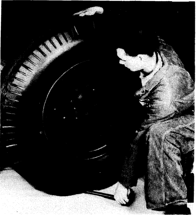
Figure 117—Removing Rear Wheel and Tire
