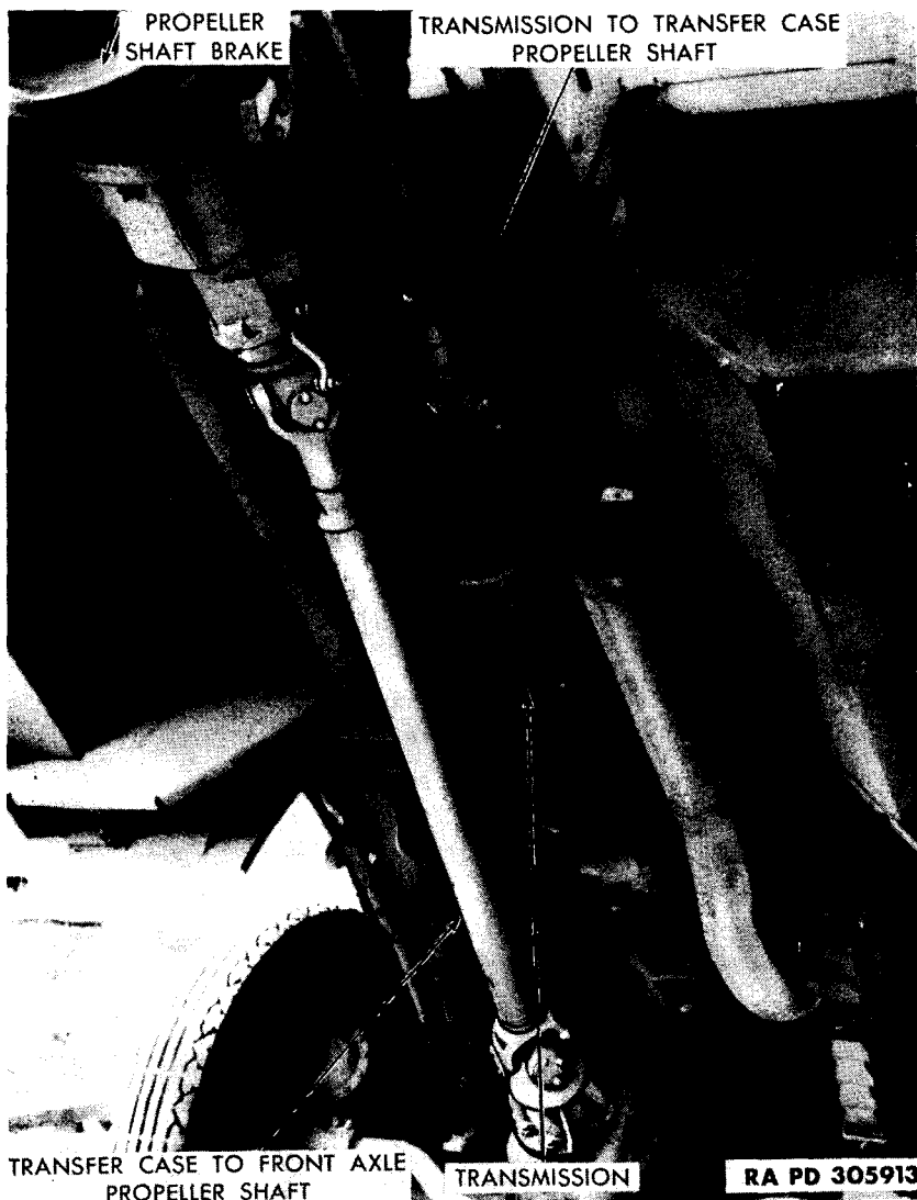
Figure 94—Propeller Shafts Installed
