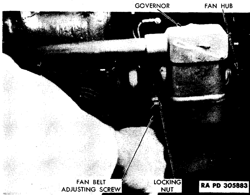
Figure 61—Unscrewing Fan Shaft Hex Nut
