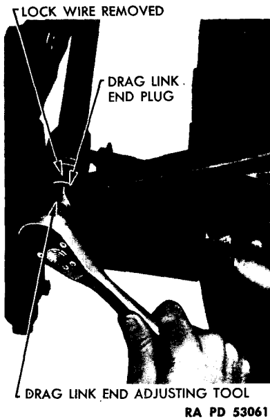
Figure 190—Adjusting Drag Link End
