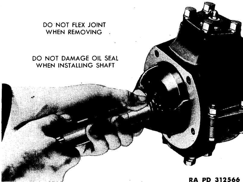
Figure 157—Removing Universal Drive Assembly
