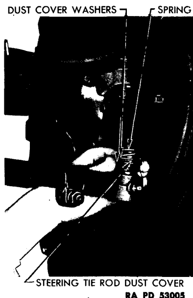
Figure 162—Installing Tie Rod Dust Cover
