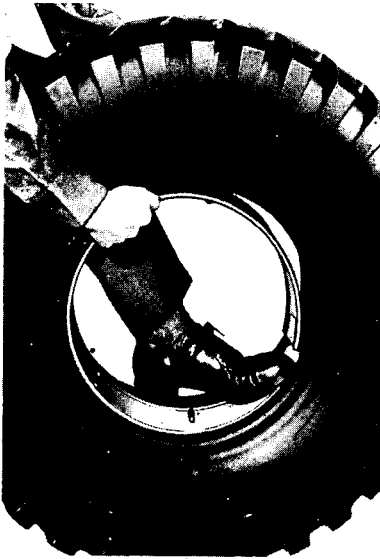
EXPANDING TIRE BEAD LOCK RING IN TIRE
