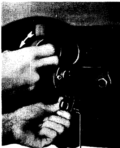
PRESS LATCH TO RELEASE JAW
