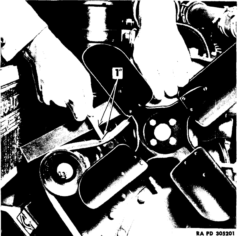
Figure 45—Fan Belt Deflection
