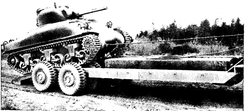
Figure 34—Using Front and Rear Tandem Winches in Unloading Recovered Tank
