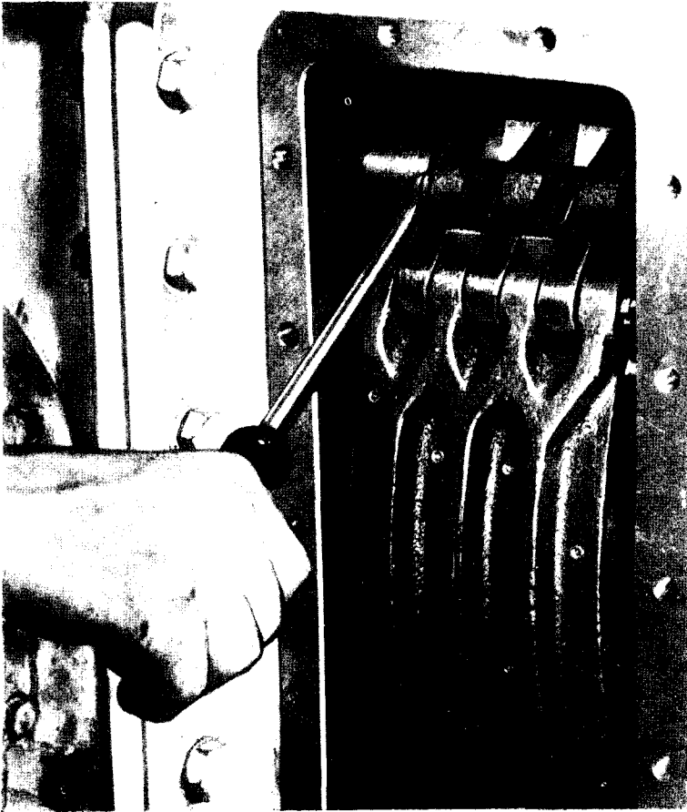
Figure 78—Removing Link Pin from Cam
