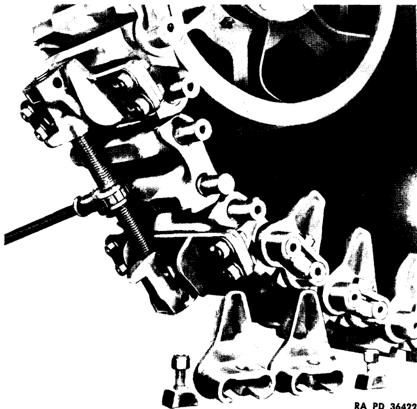
Figure 88—Replacing Dead Track Block
