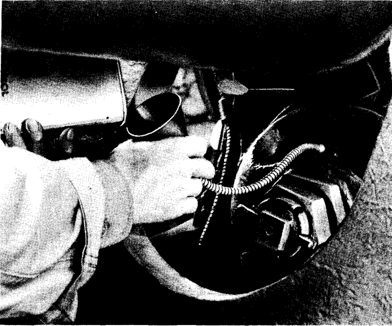
Figure 28—Filling Recoil Cylinder M1903 Carriage
