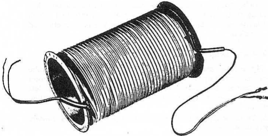
Figure 42—Rear Spacer Tube Wound With Wire
