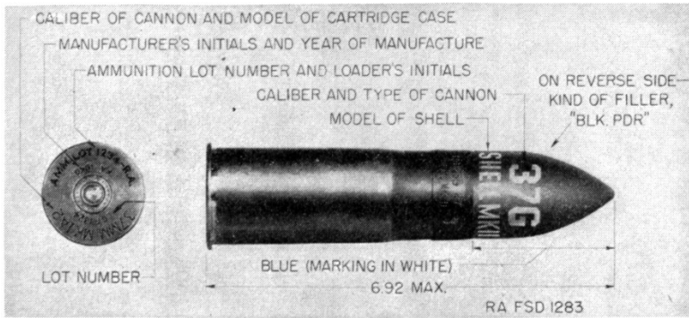
FIGURE 55.—Shell, fixed, practice, Mk. II, w/fuze, practice, M38, 37-mm gun, 1916.
