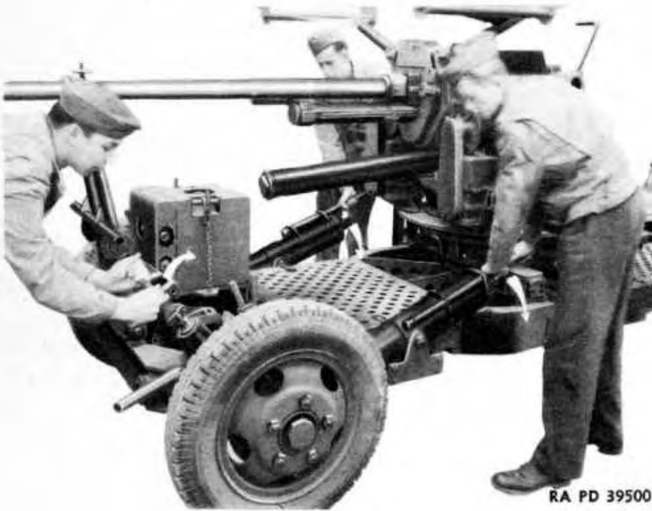
Figure 41 — Lowering Rear of Carriage to Firing Position
