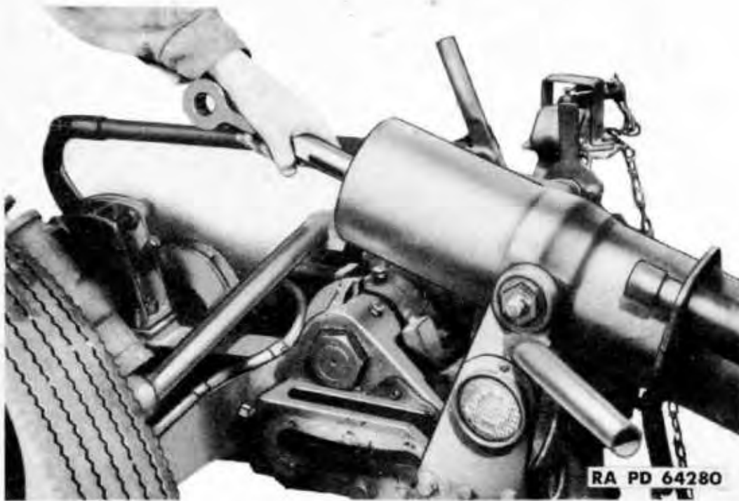
Figure 134 — Removing Counterpoise Rod
