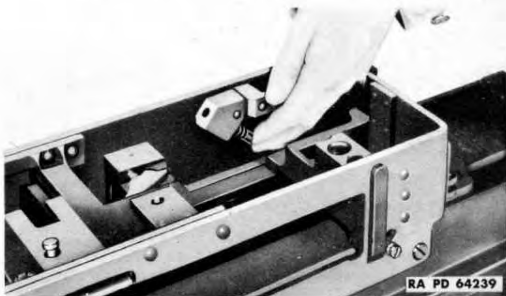
Figure 110 — Removing Feed Lever Spring Plunger and Springs
