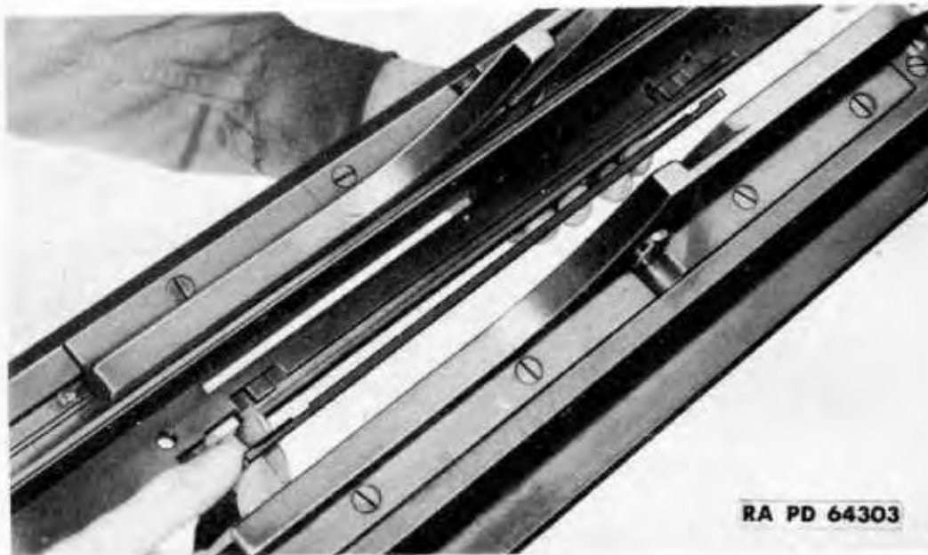
Figure 119 – Removing Trigger Bar
