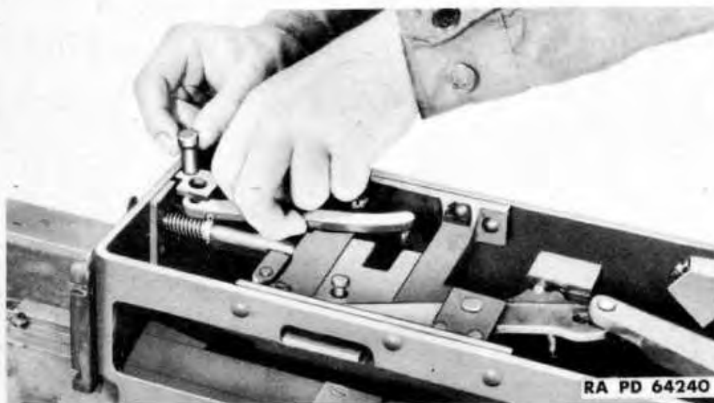
Figure 107 — Removing Feed Slide Return Lever
