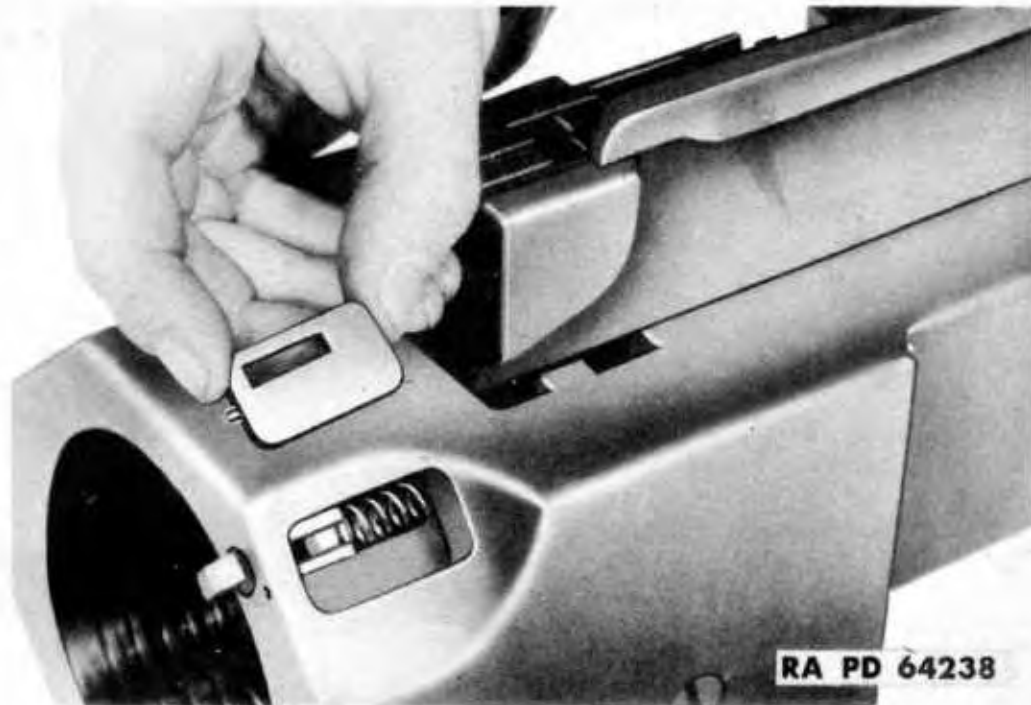
Figure 97 — Removing Tube Lock Plate Assembly
