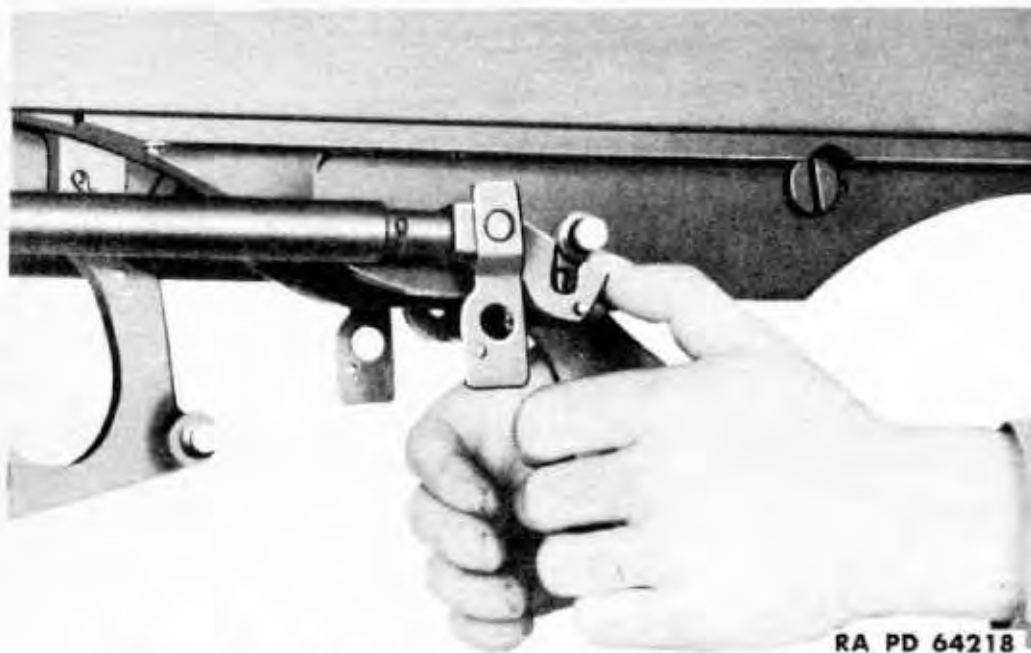
Figure 68 – Unhooking Driving Spring Assemblies
