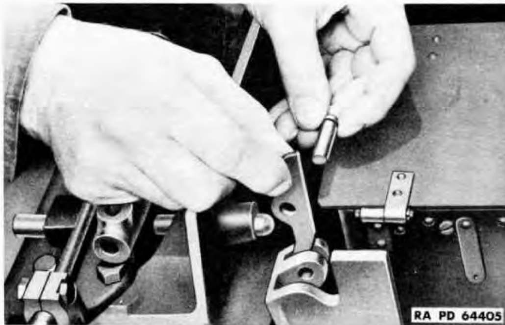
Figure 64 — Removing Foot-firing Trunnion Arm
