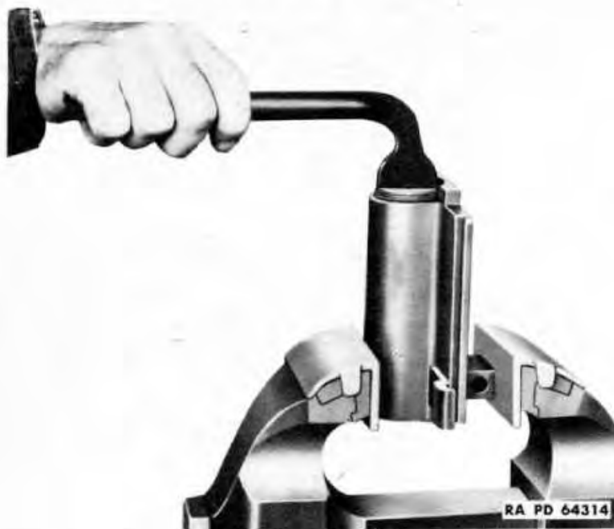
Figure 70 – Removing Buffer Adjusting Screw
