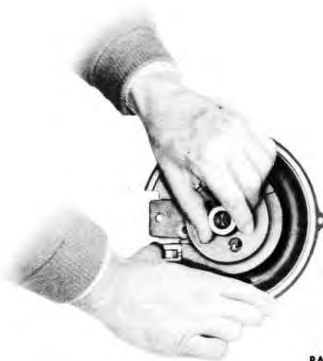
Figure 89 – Engaging Rack to Ratchet Segment
