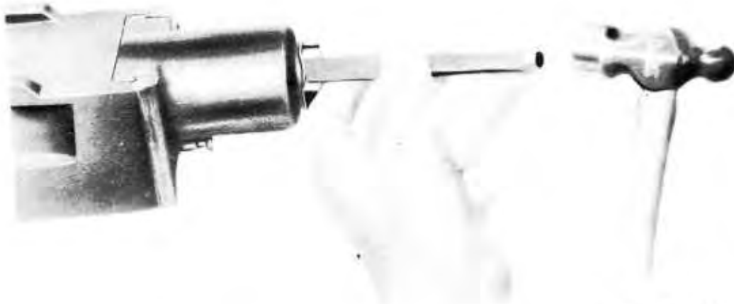
Figure 68 — Straightening the Retainer
