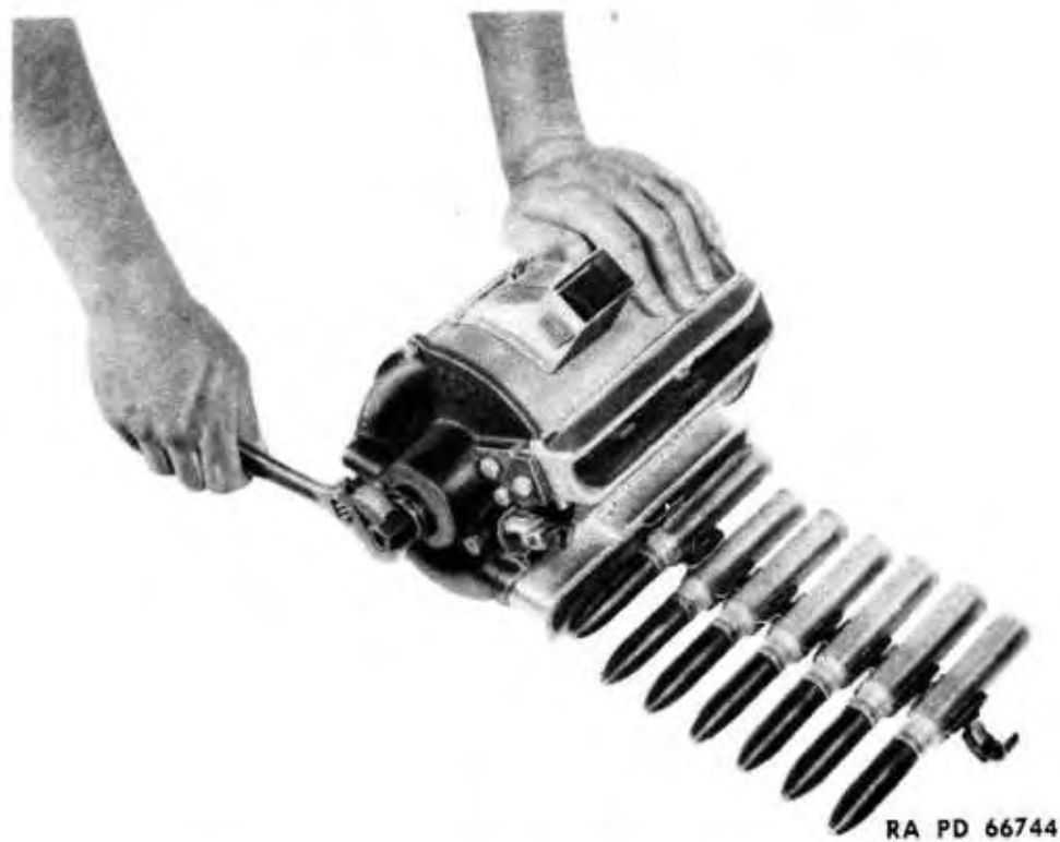
Figure 57 — Loading R.H. Feed Mechanism
