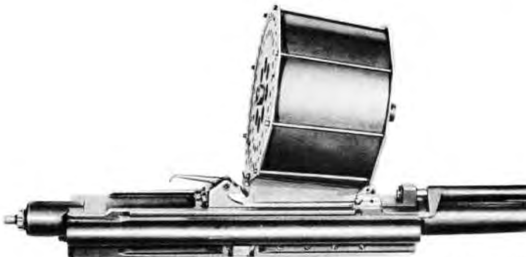
Figure 67 – Loaded Magazine in Position on Gun
