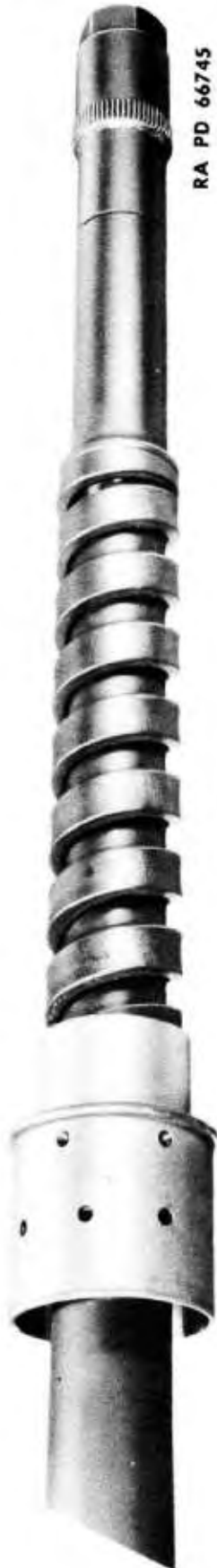
Figure 34 — Typical Installation of 20-MM Adapter M7 with Thread Protector
