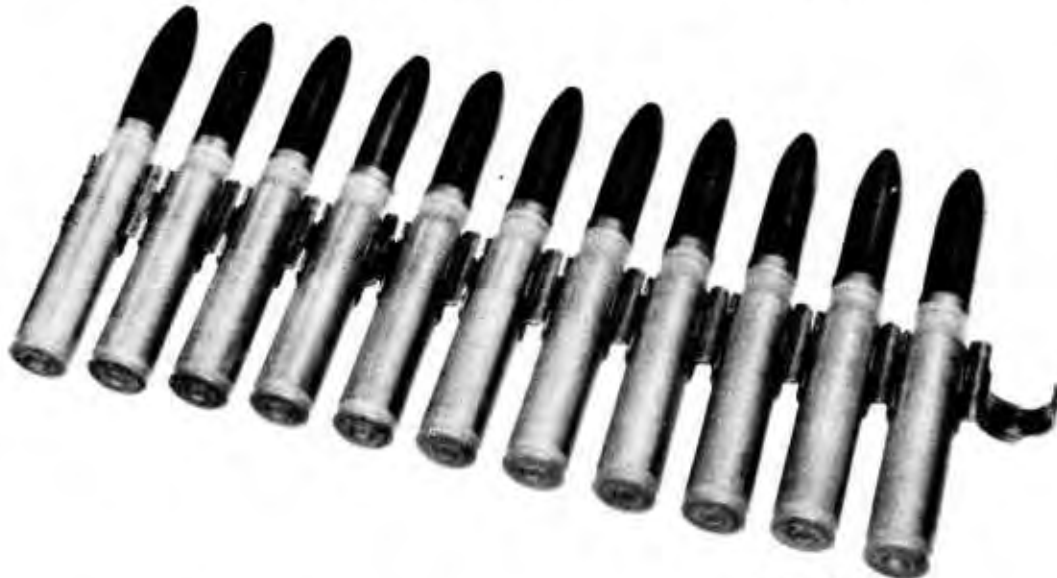
Figure 53 – 20-MM Rounds in Links for L.H. Feed
