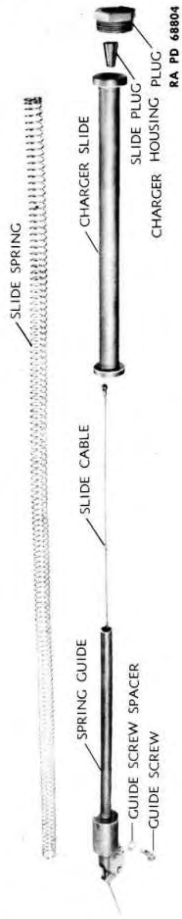
Figure 42 — Manual Charger 20-MM M2 — Installation
