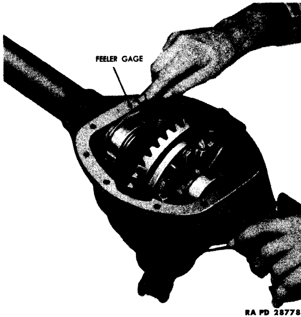
Figure 69—Checking Clearance Between Differential Case and Bearing
