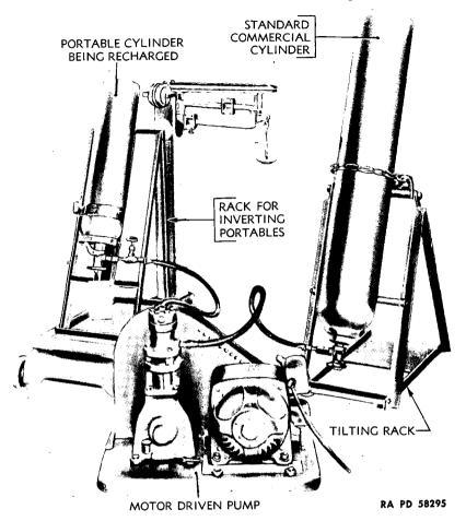
Figure 5 — Charging CO<sub>2</sub> Fire Extinguisher With A Transfer Unit
