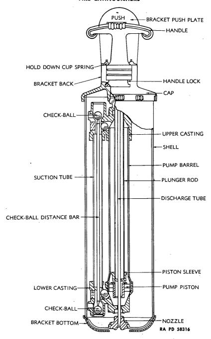
Figure 28 — Fire Guard Fire Extinguisher — Sectionalized
