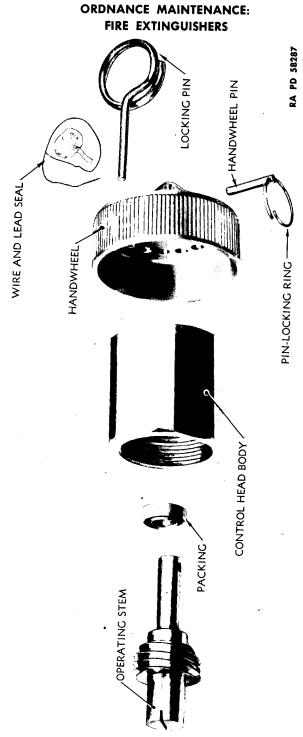
Figure 22 — Kidde-Lux Handwheel Control Head — Disassembled
