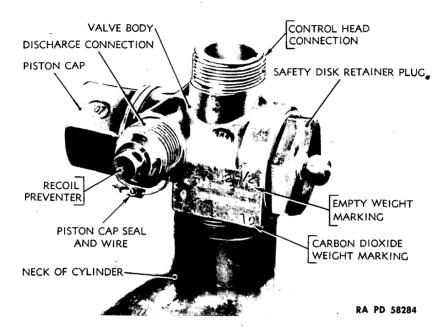
Figure 19 — Kidde-Lux Valve (7½- And 10-Pound Extinguishers)
