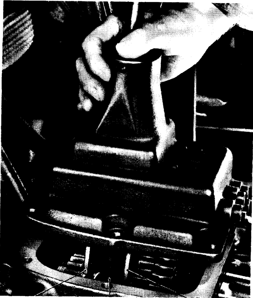
THIRD AND HIGH REVERSE SHIFTING FIRST AND SECOND SHIFTING FORK FORK SHIFTING FORK
