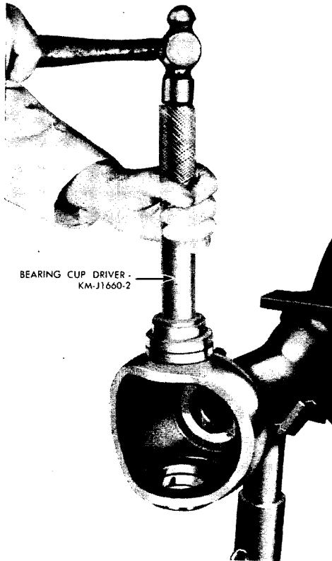
Figure 8—Installing Steering Knuckle Bearing Cup
