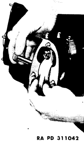
Figure 31 — Removing Rocker Arm
