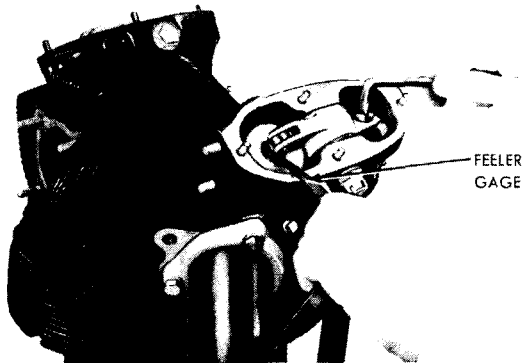
Figure 67 – Adjusting Valve Clearance, Using Gage 5A2281
