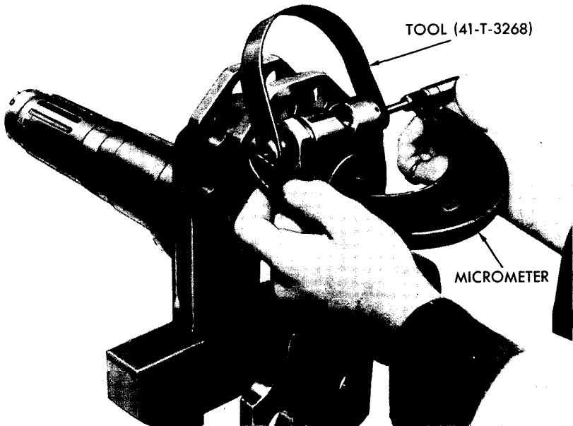
Figure 94 – Measuring Crankcheek Cap Screw Stretch
