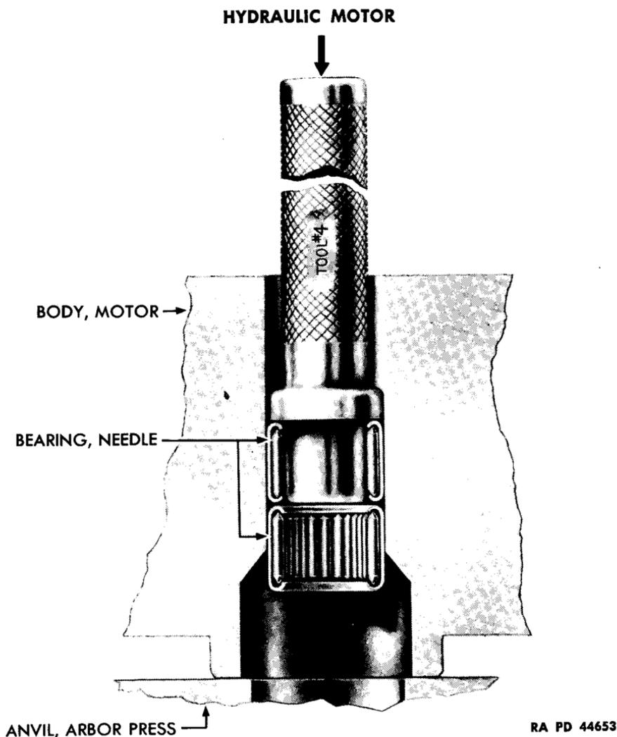
Figure 48 – Removal Of Shaft Needle Bearing From Motor Body
