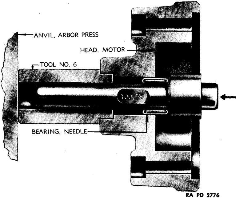
**Figure 49 – Installing Shaft Needle Bearing In Motor Head**
