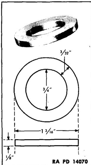
Figure 83 – Special Tool Washer
