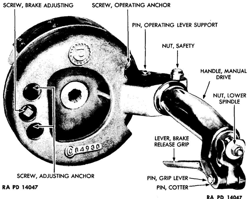
**Figure 60 — Bottom View Of Brake Mechanism Assembly**
