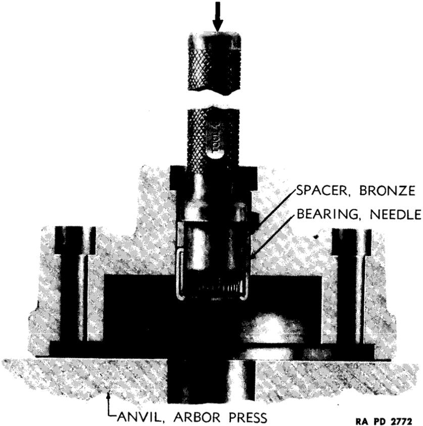
Figure 47 — Removing Shaft Needle Bearing And Spacer From Motor Head
