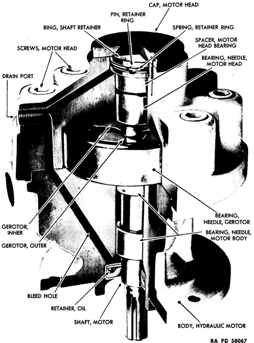
Figure 46 – Cutaway View of Hydraulic Motor
