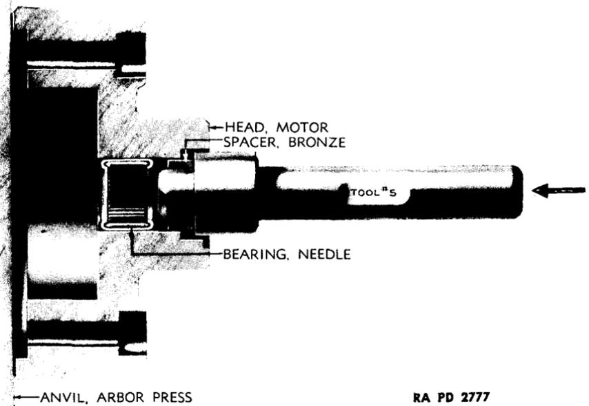
**Figure 50 – Installing Bronze Spacer In Motor Head**
