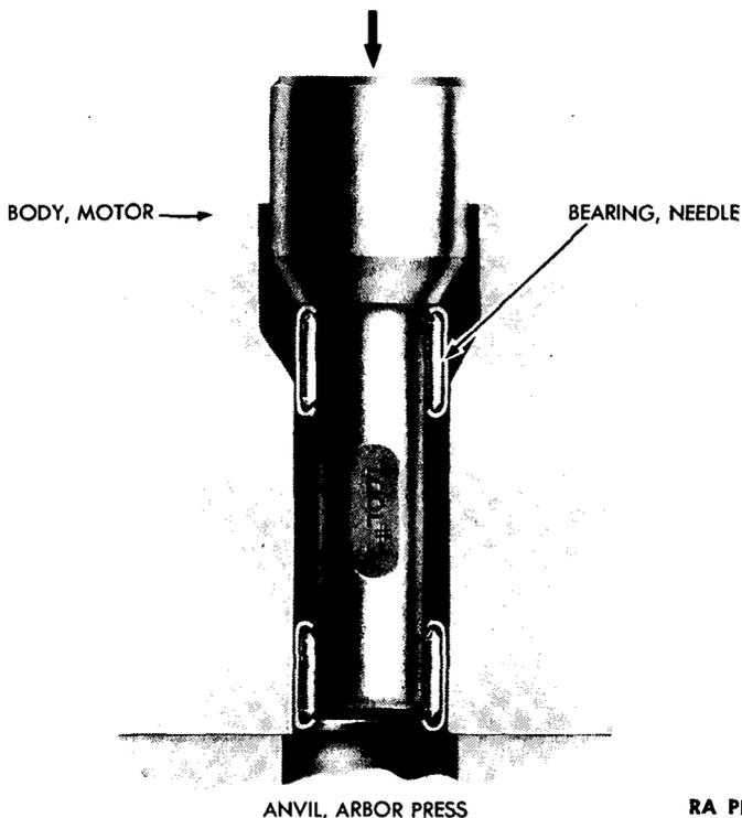
**Figure 52 – Installing Shaft Outer Needle Bearing In Motor Body**
