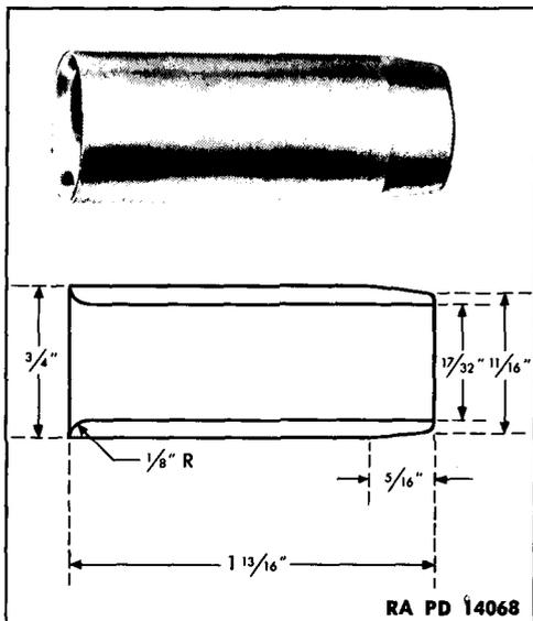
Figure 82 – Hydraulic Motor And Pump Shaft Assembly Tool
