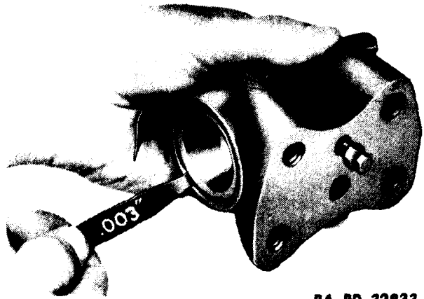
Figure 67 – Checking Fit of Piston in Cylinder Bore
