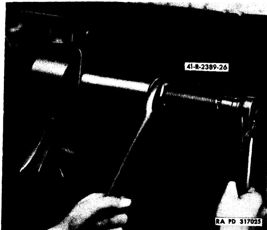
Figure 19 — Pulling Spring Shackle Pin
