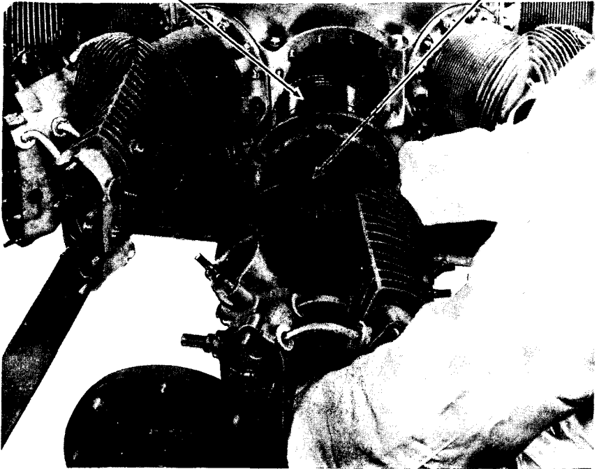
FIGURE 42—Lifting off the cylinder.
