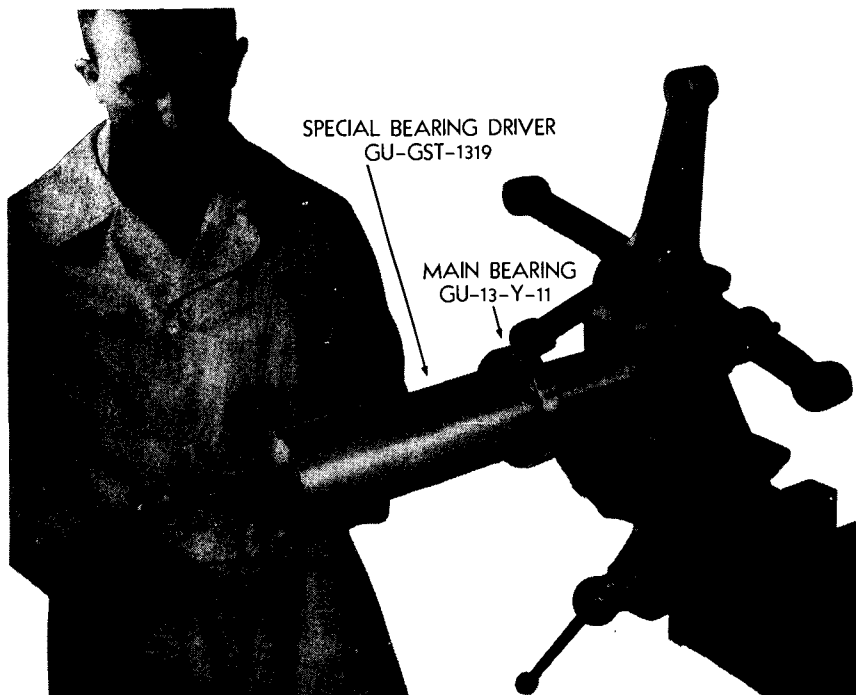
FIGURE 101—Driving main bearings onto the crankshaft. RA PD 6616
