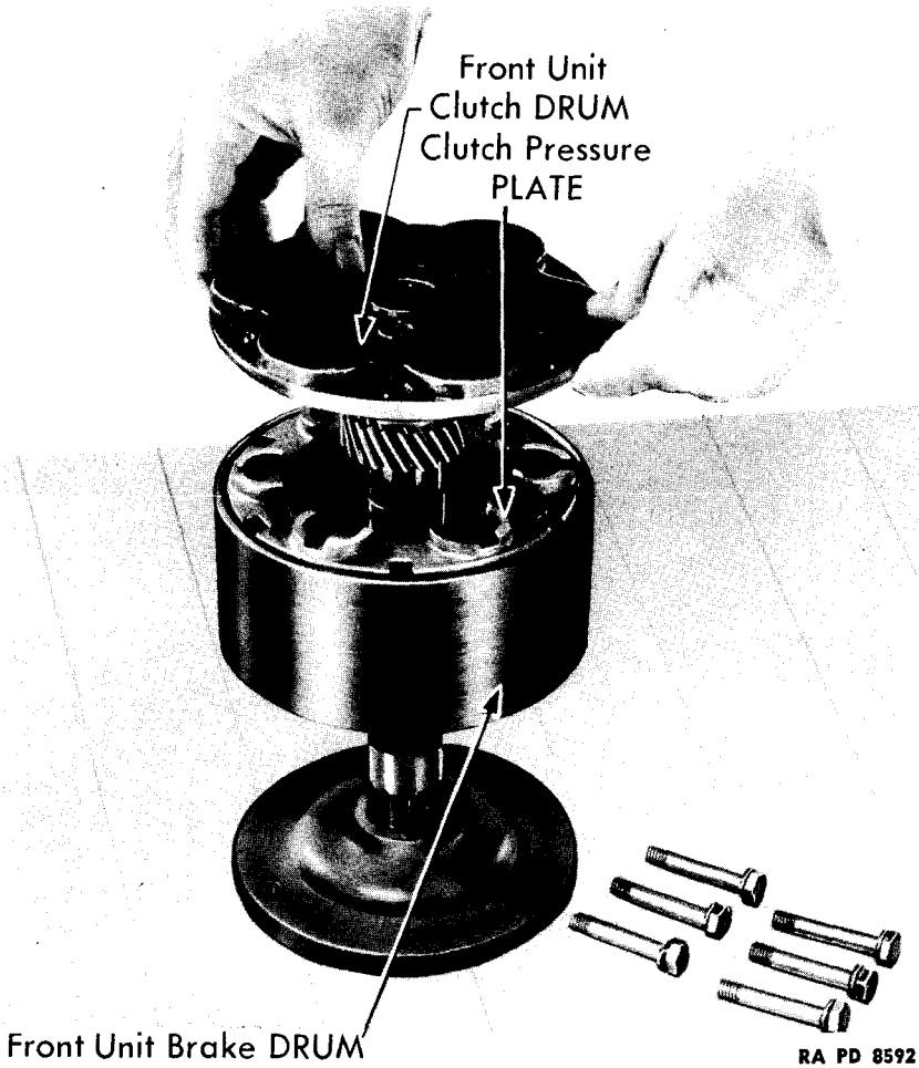
Figure 95 — Removing Front Unit Clutch Drum
