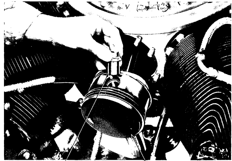
Figure 53 — Loosening Cylinder Attaching Nuts
