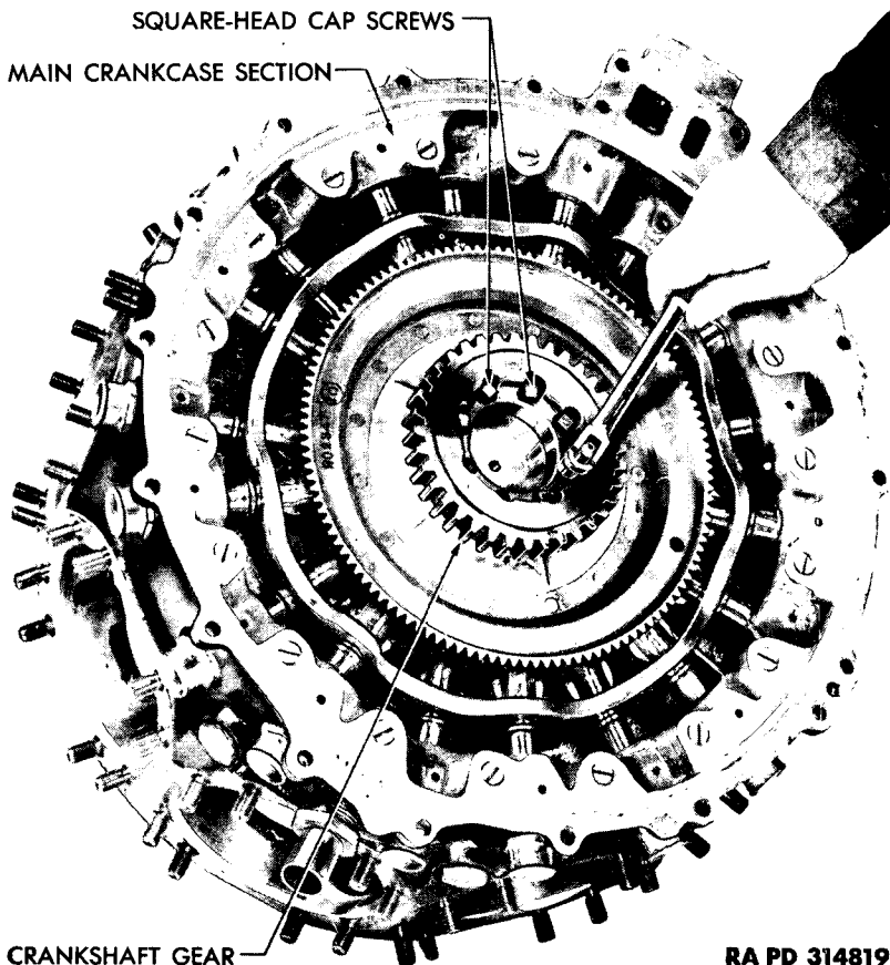
Figure 210 – Tightening Crankshaft Gear Retaining Screws
