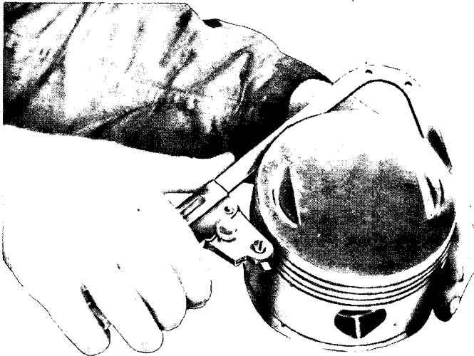
Figure 110 – Cleaning Piston Ring Grooves with Ring Groove Cleaner 41-C-2155
