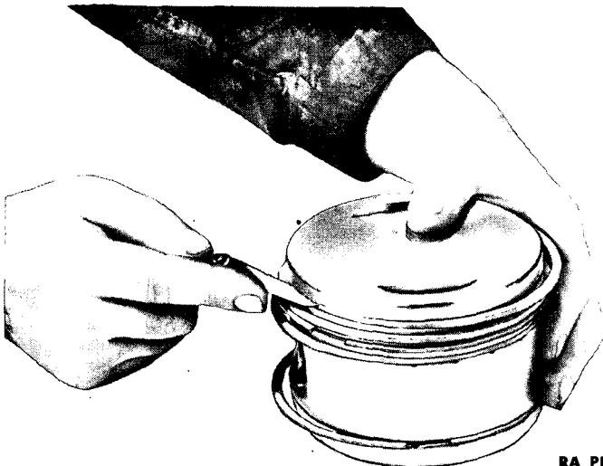
Figure 112 – Measuring Piston Ring Side Clearance Using Gage 41-G-400
