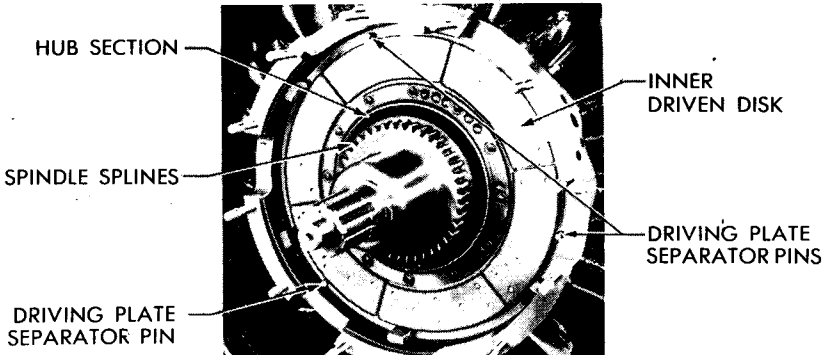
3. INNER DRIVEN DISK IN POSITION
