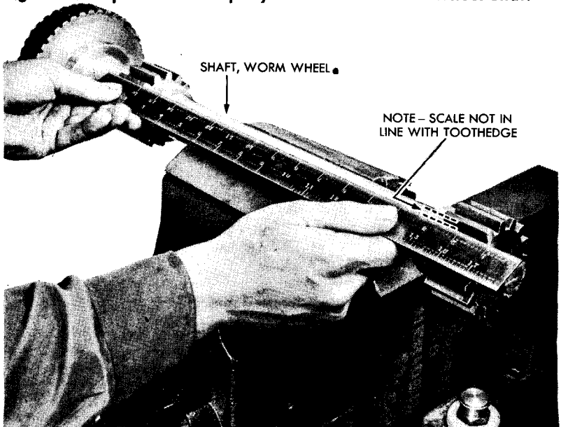
Figure 84 — Spur Pinion Properly Mounted on Worm Wheel Shaft
