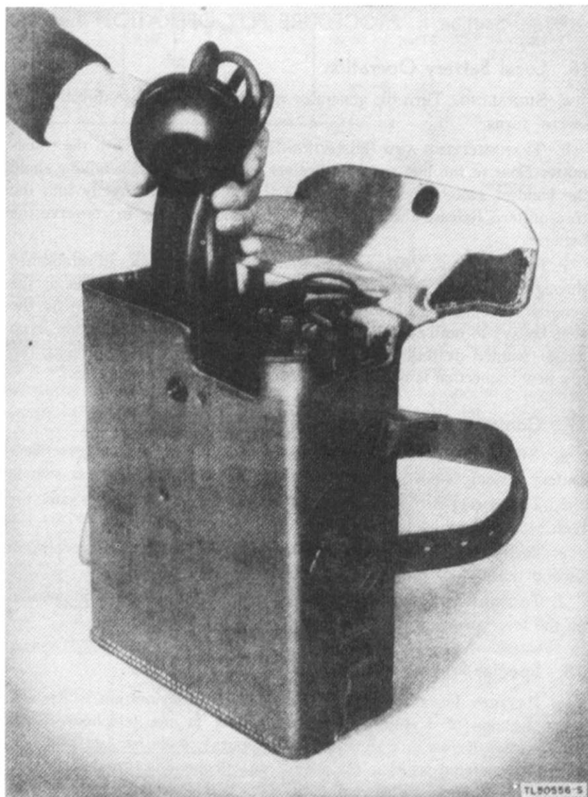
Figure 19. Replacing handset in compartment of telephone case
