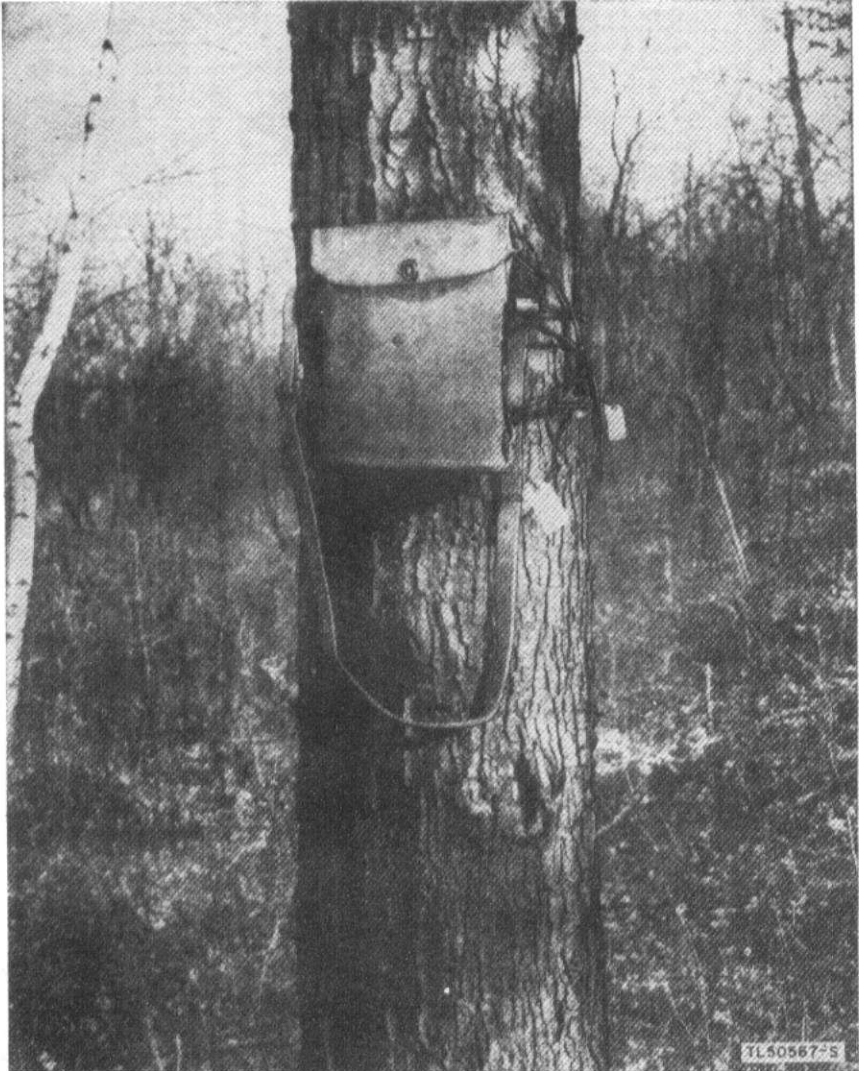
Figure 12. Telephone EE-8-A suspended from tree trunk,
