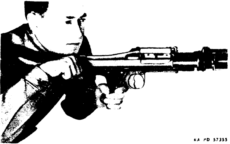
Figure 29 – Cocking Handle in Rearmost Position – Gun Cocked
