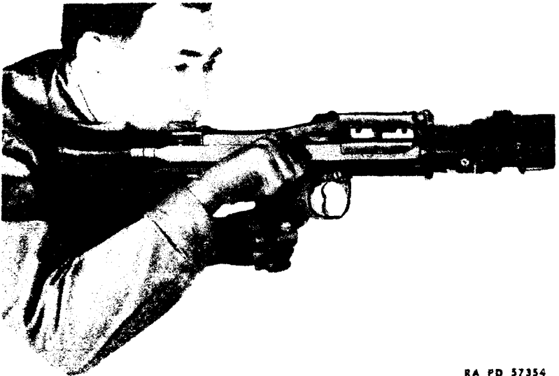
Figure 30 – Cocking Handle in Forward Position – Gun Cocked
