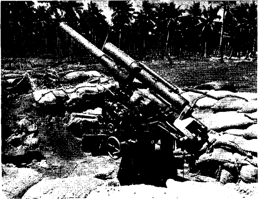
Figure 62.—Model 10 (1921) 3-inch (76.2-mm) naval dual-purpose gun captured on Guadalcanal.
