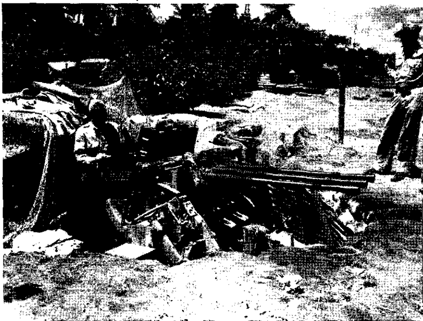
Figure 67.—25-mm automatic cannon, triple mount.
