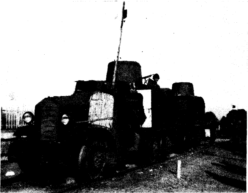
Figure 74.—“Sumida” armored car, fitted with flanged steel tires for rail travel. Note that two cars have been coupled back to back, permitting rapid movement in either direction.
