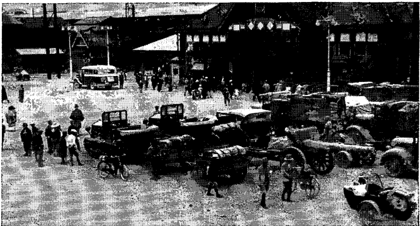
Figure 3.—Part of a motorized 105-mm gun battery. (The tractors are 4-ton Model 94 Sumidas; one draws two Model 92 gun caissons, each holding 24 rounds, the other a Model 92 105-mm gun. The touring car is a Model 1929 Buick. Beyond the Buick is a Model 94 truck chassis fitted as a battery detail vehicle.)
