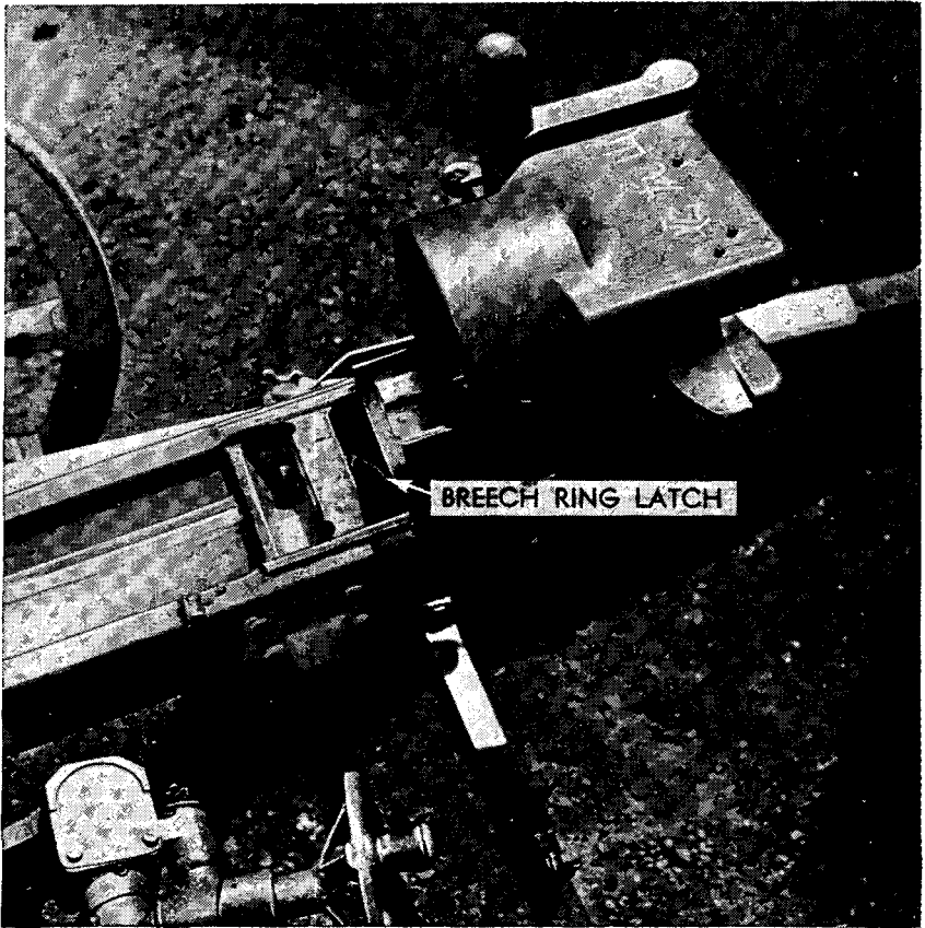
Figure 93. Fourth step: (2) removal of the breech.
