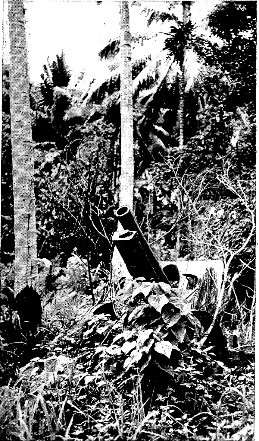
Figure 62. Model 96 (1936) 150-mm howitzer emplaced in the jungle. The tube is in full recoil.
