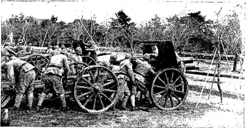
Figure 53. Assembly of Model 4 (1915) 150-mm howitzer: placing tube in battery. The second man from the left is using the winch on the side of the rear trail section to pull the tube over the removable rails to the slides.
