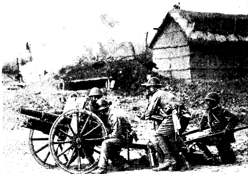
Figure 147.—Gun crew of Model 41 (1908) 75-mm mountain (infantry) gun in action. (Note the method of moving the trail.)
