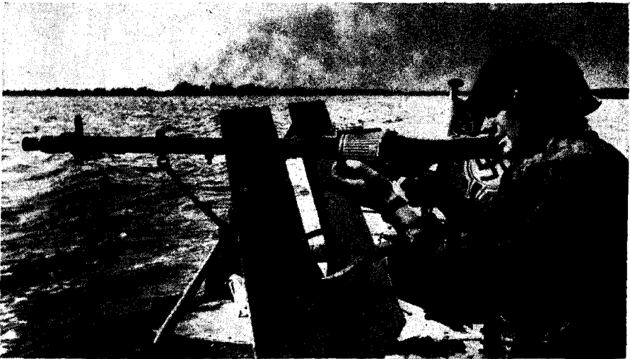
Figure 38.—M.G. 34 in action on boat, showing protective shield and drum feed.
