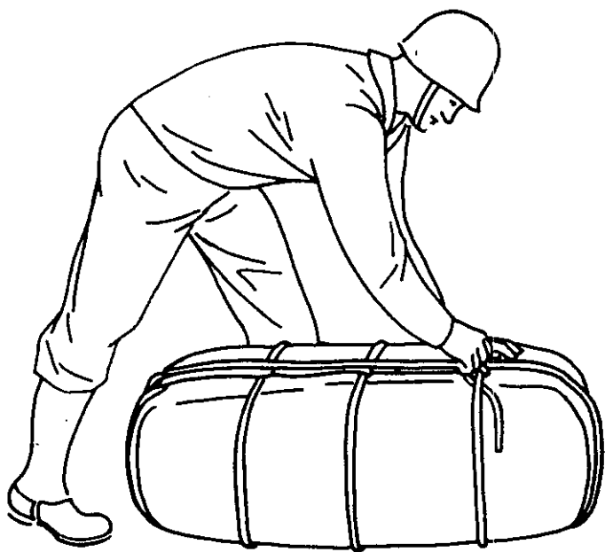
FIGURE 17. Tying off .lair rope with sliding clove hitch.
