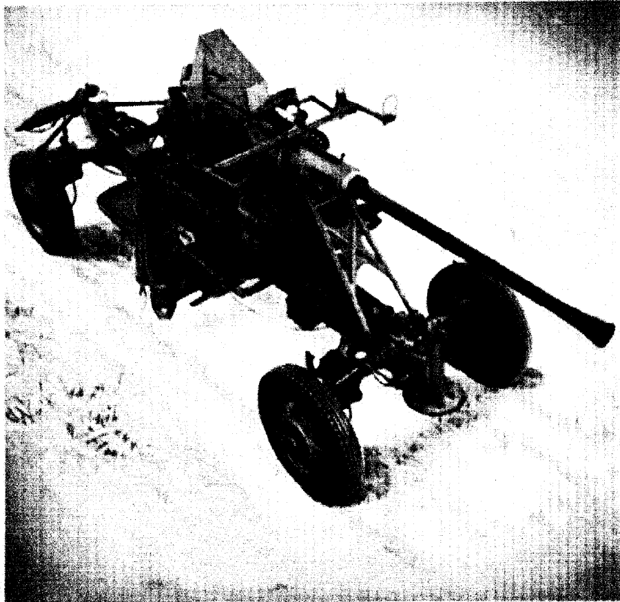
40 mm AUTOMATIC A. A. GUN, M1, ON CARRIAGE, M2A1, IN TRAVELING POSITION
