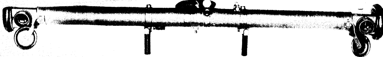
1-METER-BASE RANGE FINDER, T16, WHICH HAS BEEN MODIFIED TO BECOME M7 AND M9A1
