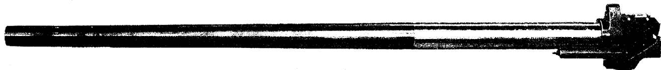
76 MM TANK GUN, M1A1. THE M1A2 DIFFERS FROM THE M1A1 ONLY IN HAVING THE MUZZLE END THREADED FOR ATTACHMENT OF A MUZZLE BRAKE
