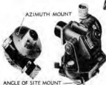
Figure 106 - Aiming Circle Components
