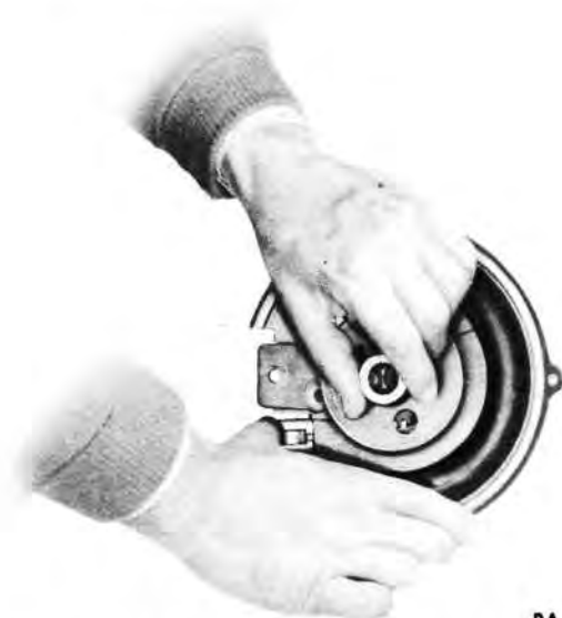
Figure 89 — Engaging Rack to Ratchet Segment
