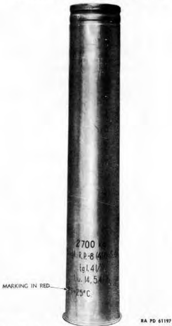
Figure 72 — German 88-mm Cartridge Case, Showing Stenciled Markings
