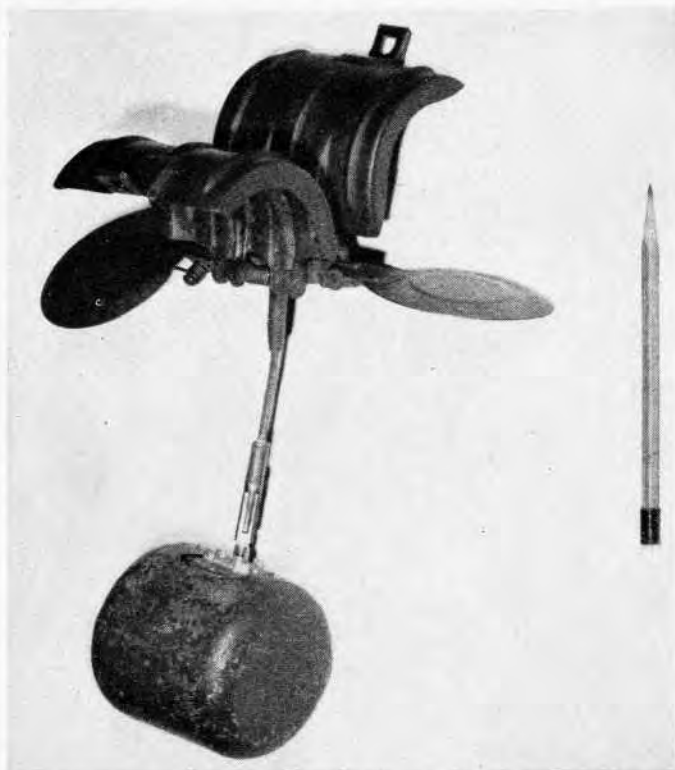
Figure 8. Danger lurks for the inquisitive in the form of the German anti-personnel bomb known as the "butterfly." Here is one of these bombs, lying as you might find it in the field.
