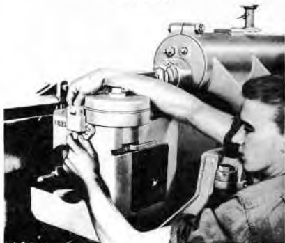
Figure 52 — Disengaging "SEMIAUTOMATIC-HAND" Catch
