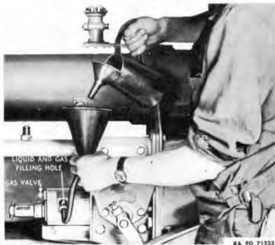
Figure 60 — Filling Rammer Cylinder with Liquid
