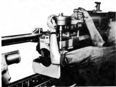
Figure 63 — Removing Breech Actuating Mechanism
