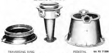
Figure 27 — Components of Pedestal Assembly
