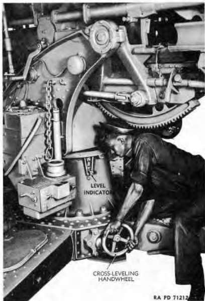
Figure 39 - Leveling Top Carriage
