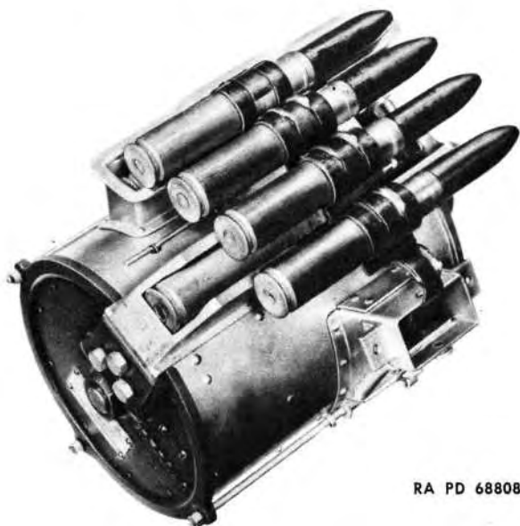
Figure 58 — Loading Feed Mechanism
