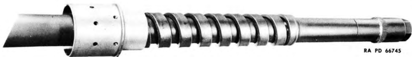
Figure 34 — Typical Installation of 20-MM Adapter M7 with Thread Protector
