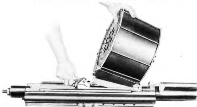
Figure 66 – Installation of 20-MM 60-round Magazine M1 on Gun
