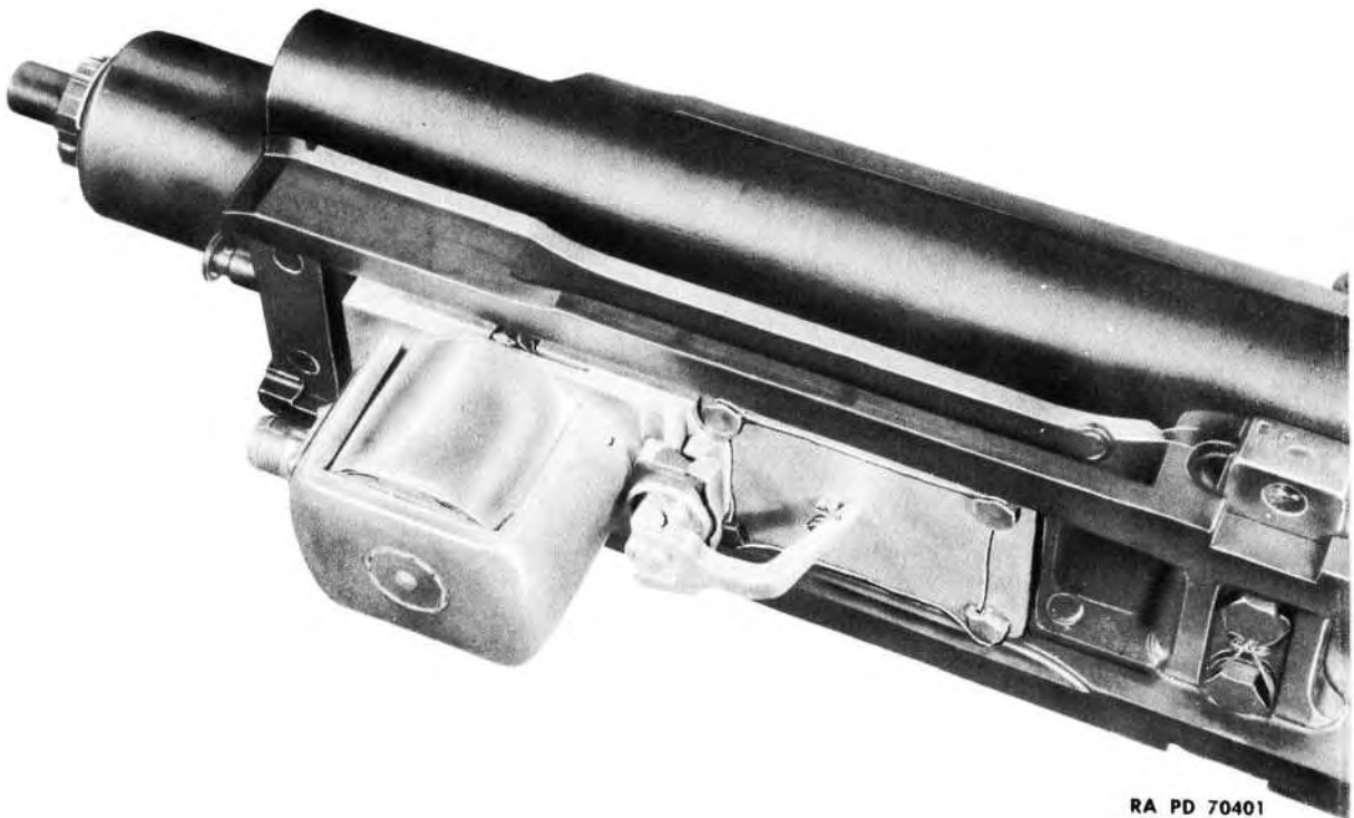
Figure 36 — Electric Trigger AN-M1 on Gun
