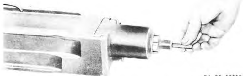
Figure 69 – Inserting the Driving Spring Assembling Tool
