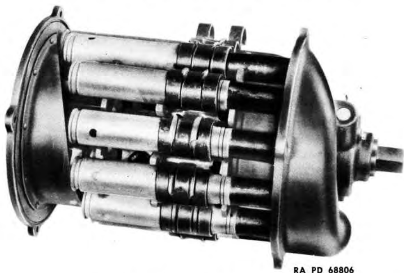
Figure 48 — Separation of Links from Rounds in 20-MM Feed Mechanism AN-M1 — Right Side View
