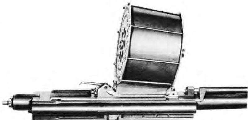
Figure 67 — Loaded Magazine in Position on Gun
