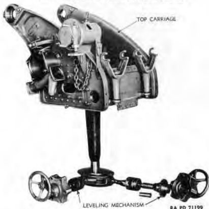
Figure 26 — Top Carriage Leveling Mechanism
