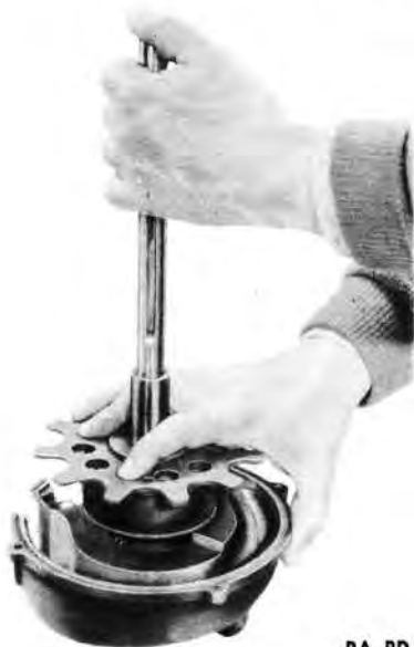
Figure 90 — Inserting Shaft into Hub
