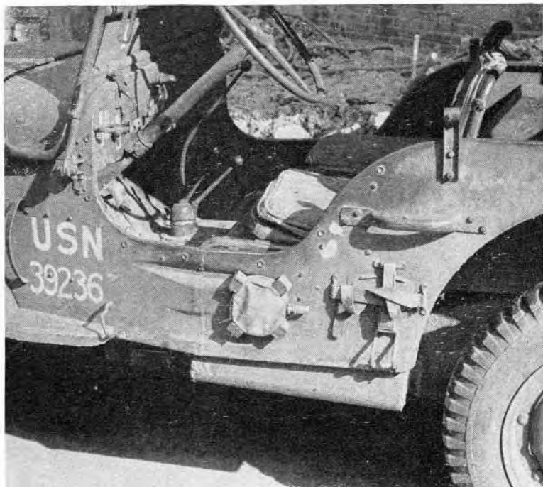
Figure 12. Antitank magnetized mine on side of jeep as enemy might place it on one of our vehicles if given a chance. When so placed as a trap, pressure is applied to ignite cap causing an explosion, within 7 seconds.
