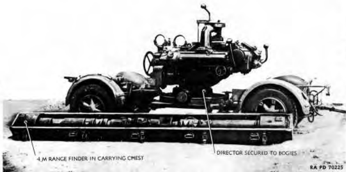
Figure 90 — Stereoscopic Director 36 (Kdo. Gr. 36) — Range Finder Removed from Director
