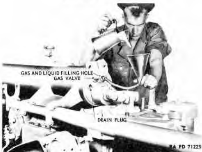
Figure 56 - Filling the Recuperator Cylinder with Liquid
