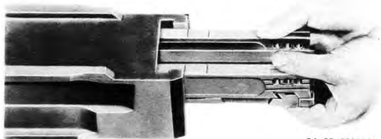
Figure 76 – Removing (or Replacing) the Breechblock
