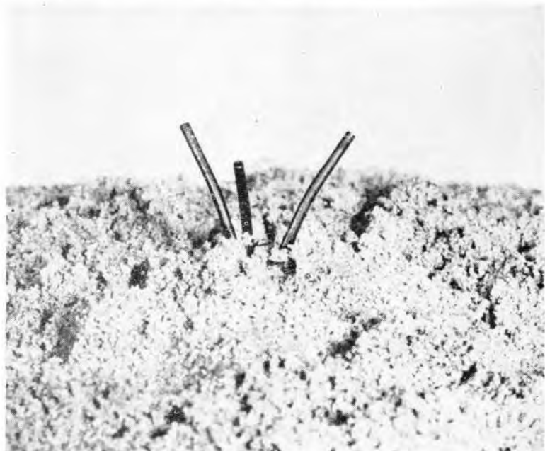
Figure 2.—"S" mine buried in ground with three-prong igniter projecting above surface. Pressure on the prongs causes explosion of mine. This is a commonly used trap. Watch out for it in shore or inland areas recently held by the enemy.
