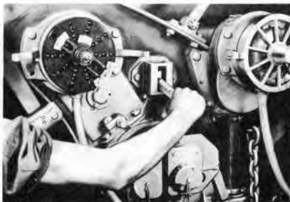
Figure 37 — Engaging Elevation Gear Clutch
