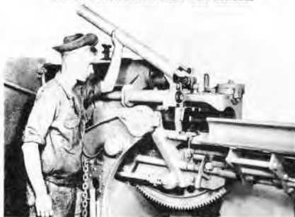
Figure 40 — Unfolding Rammer Guard
