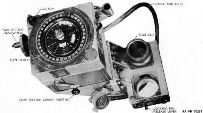
Figure 102 — Fuze Setter — Close-up, Showing Cover Removed and One Fuze Cap Disassembled
