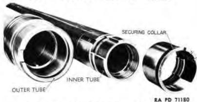
Figure 7 — Method of Securing Inner and Outer Tubes
