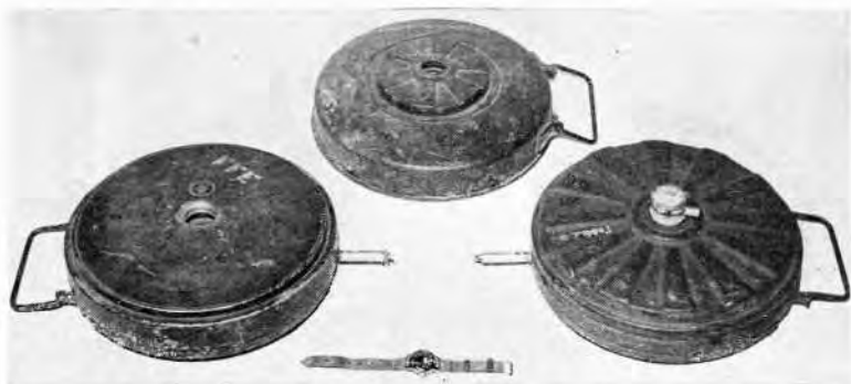
Figure 5. Tank mines used by the Germans. Watch for these on roads and along the sides of roads. Pull igniters of two mines in foreground are connected so that moving of either mine will set off both of them. Pressure igniters have been removed from two of the mines.
