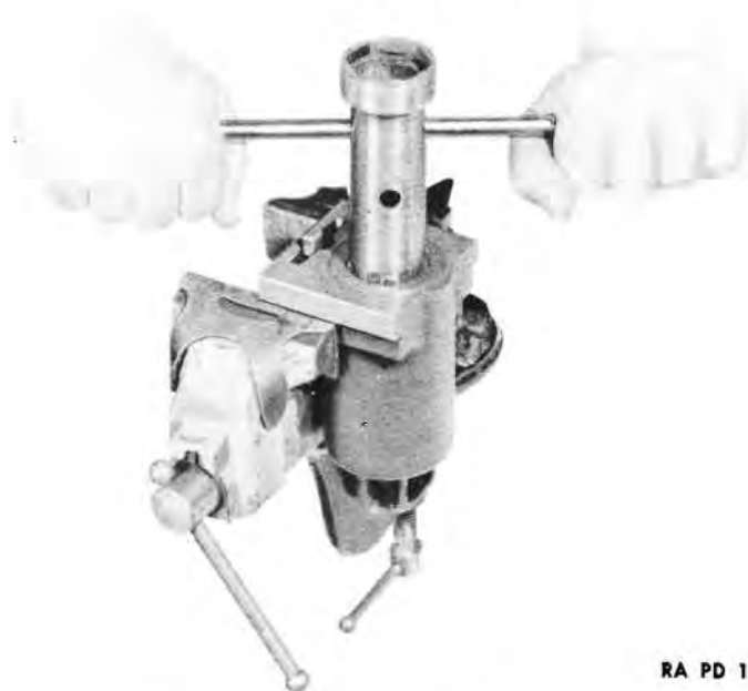
Figure 71 — Unscrewing the Rear Buffer Sleeve
