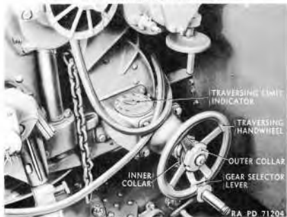
Figure 31 — Traversing Limit Indicator
