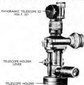
Figure 86 — Panoramic Telescope 32 (Rbl. F. 32) in Telescope Holder
