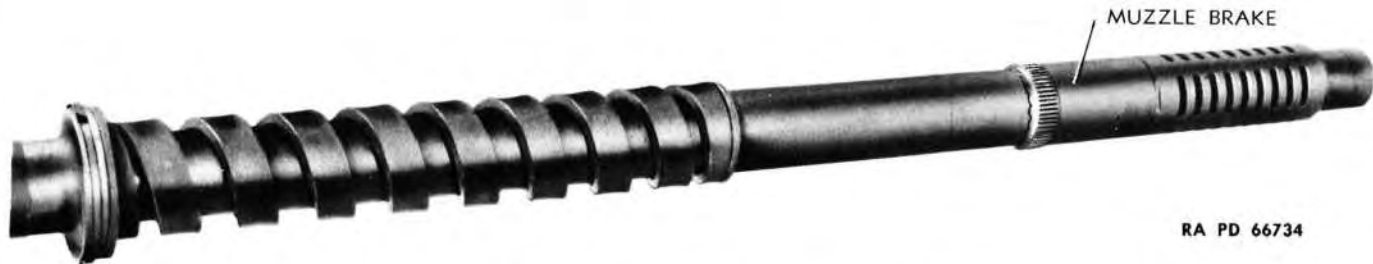
Figure 32 — 20-MM Adapter M7 with Muzzle Brake
