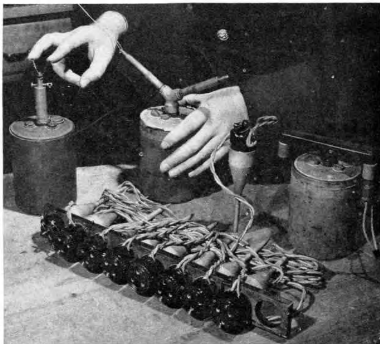
Figure 3. Three types of firing devices for "S" mines.
