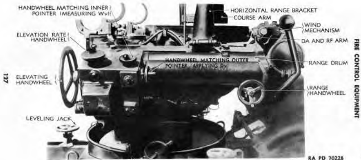
Figure 93 — Stereoscopic Director 36 (Kdo. Gr. 36) — View of Range Drum
