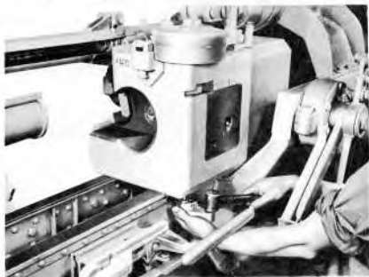
Figure 62 — Removing Breech Operating Crank
