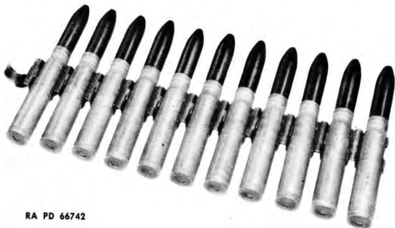
Figure 51 – 20-MM Round in Links for R.H. Feed
