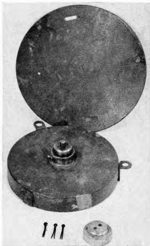
Figure 7. CVP is a Hungarian anti-tank mine used by the Germans. It can also be set as an antipersonnel mine. It is generally placed along roadways and in mine fields. Downward pressure at any point on the cover (thrown back in picture) will cause fuse to operate.
