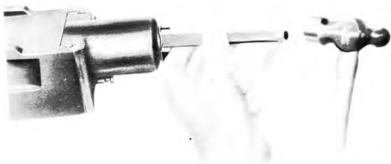
Figure 68 – Straightening the Retainer
