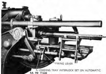
Figure 53 — Shell Partially Rammed
