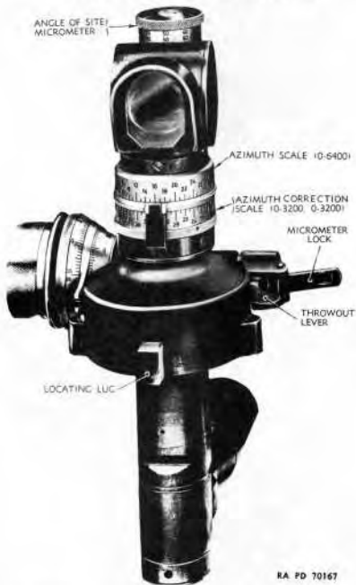
Figure 88 — Panoramic Telescope 32 (Rbl. F. 32) — Front View
