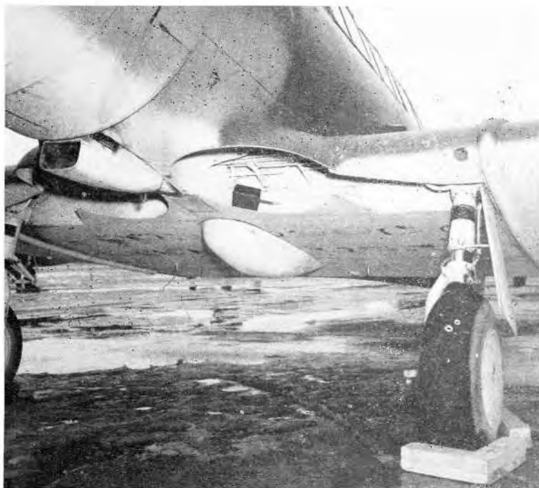
Figure 20. This plane has a tension release device attached to the landing gear and connected to a concealed explosive container. Device is fired, after take-off, as wheels are folded. The Japs placed traps in similar fashion on American planes at Guadalcanal.
