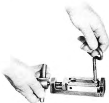
Figure 81 — Sear Block Group in Position in the Tool
