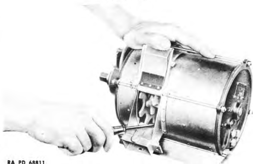
Figure 65 — Removal of Last Round
