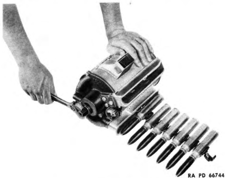
Figure 57 — Loading R.H. Feed Mechanism
